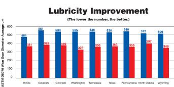
The ASTM D975 diesel fuel standard specifies a wear scar below 520 µm in ASTM D6079 testing, while the Engine Manufacturers Association (EMA) specifies a wear scar below 460 µm. Testing reveals AMSOIL Diesel Injector Clean provides significant lubricity improvement in diesel fuels found across the U.S., delivering improved wear protection.
