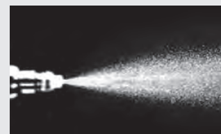
Injector spray pattern after P.i. treatment.
