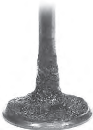
Intake Valve before P.i. Treatment
